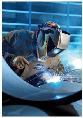
form a permanent bond. Because of its strength, welding is used in shipbuilding, automobile manufacturing and repair, aerospace applications, and thousands of other manufacturing activities. Welding also is used to join beams in the construction of buildings, bridges, and other structures and to join pipes in pipelines, power plants, and refineries.
