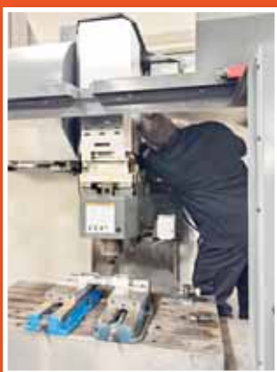
Computer Numerical Control (CNC) Machine Installation
